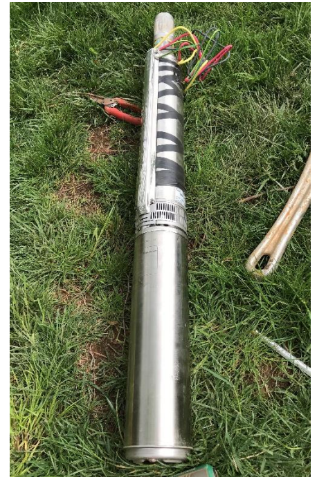
New assembly: 2 HP motor on the bottom, then the 25 gpm pump, topped by a stainless steel check valve.
