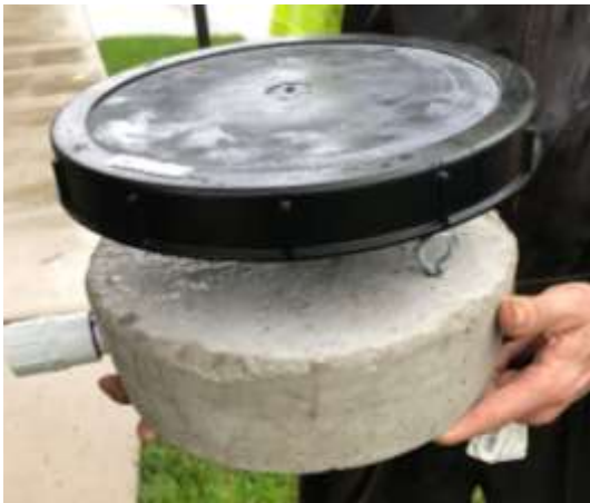
One of three air diffusers that sit on the pond bottom, fed by self-weighted plastic tubing. Pond 1 diffusers are identical.
