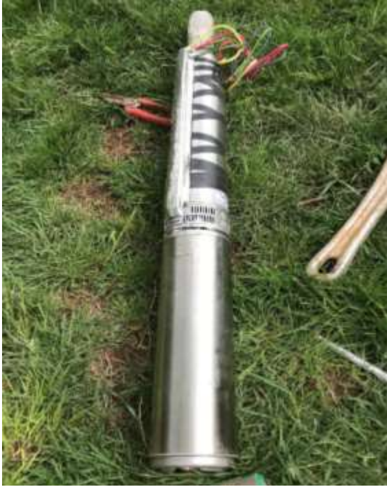
The Goulds well pump (top) and 2 HP Franklin Electric motor (bottom) prior to installation in May 2021.
