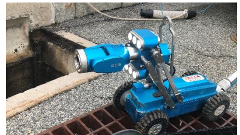
Camera/crawler in position on Sloan Road
