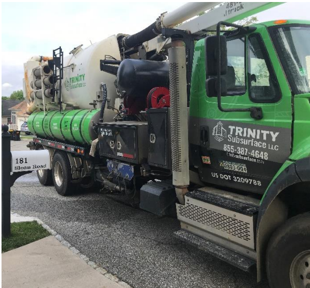
The hydro-vac truck pumps high pressure water, uses a vacuum system to extract it and has tanks to store both the clean and spent water.
