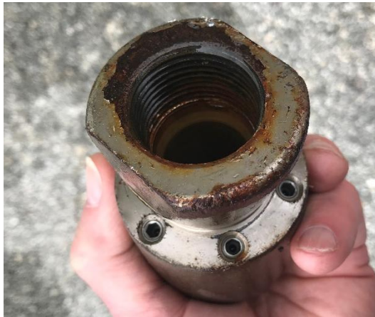
The high pressure cleaning head has rear-facing nozzles that propel the hose forward as the pipe interior is cleaned.
